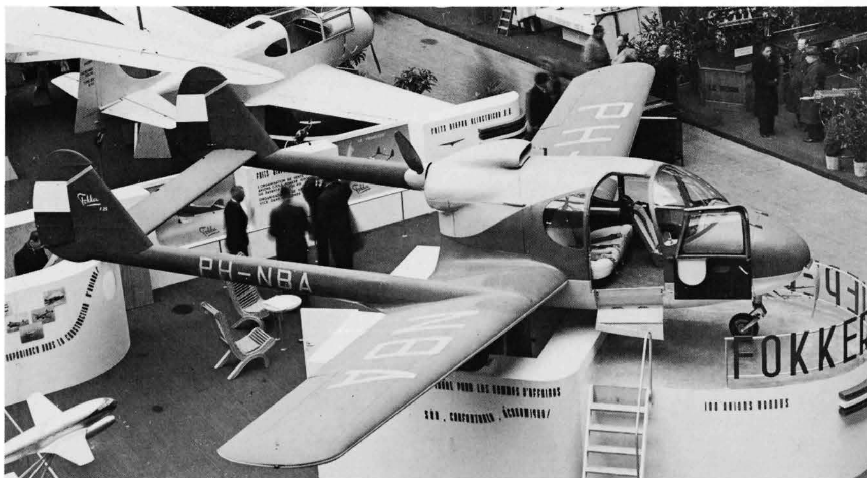
Above: The Fokker F.25 Promoter four-seat twin boom cabin monoplane with retractable tricycle undercarriage and a 190 hp Lycoming O-435-A flat six engine with a two position variable pitch pusher propeller. The prototype PH-NBA c/n 6066 was rushed through just
