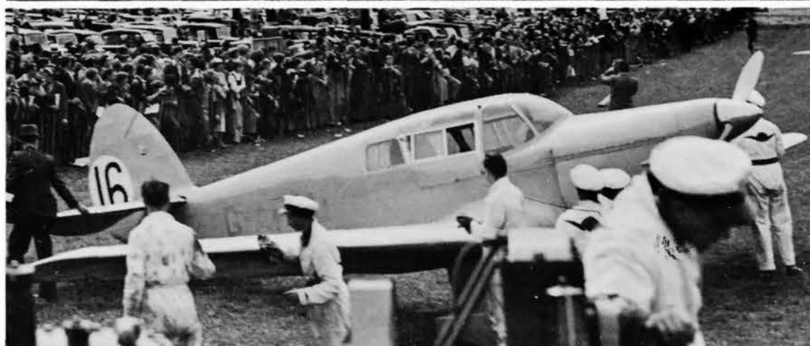
The lower photograph depicts the same aircraft as it appeared as No.16 at the 1938 King's Cup. By this time the windscreen had been changed to the rounded type fitted as standard to the Vega Gull Series II.
