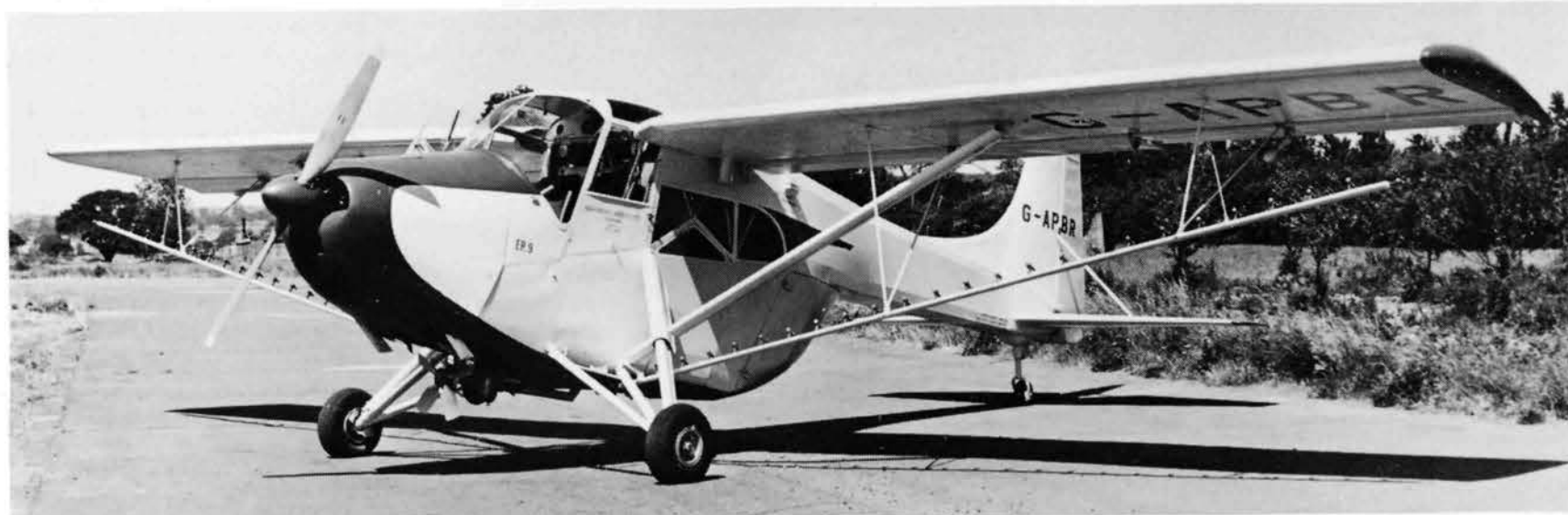
Above: G-APBR c/n 28, ex G-43-7, while still with Edgar Percival Aircraft awaiting sale, is fitted out with spray bars under the wings and a fan-driven pump under the nose. This allowed a 90-foot wide swath to be sprayed from a 170 gallon hopper in the fuselage. (Aeroplane via Jack Meaden)
