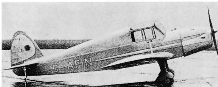
Above: The two-seat Chrislea Airguard had a wingspan of 35ft 9in. Structure was spruce with plywood covering and all-up weight was 1300 lbs. (Aeroplane via Jack Meaden)
