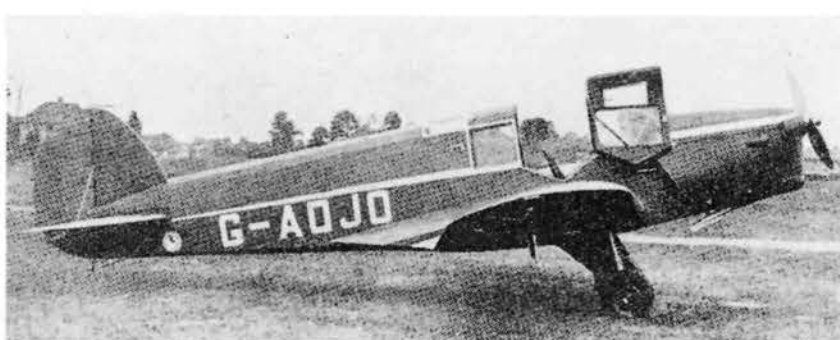
Below: G-ADJO B.A. Eagle 2 c/n 122 was purchased by entrant Major Hargreaves in 11.36. Its 130 hp Gipsy Major engine gave it a maximum speed of 148 mph but, piloted by Tommy Rose, it failed to gain a place. (Both: Aeroplane via Jack Meaden)
