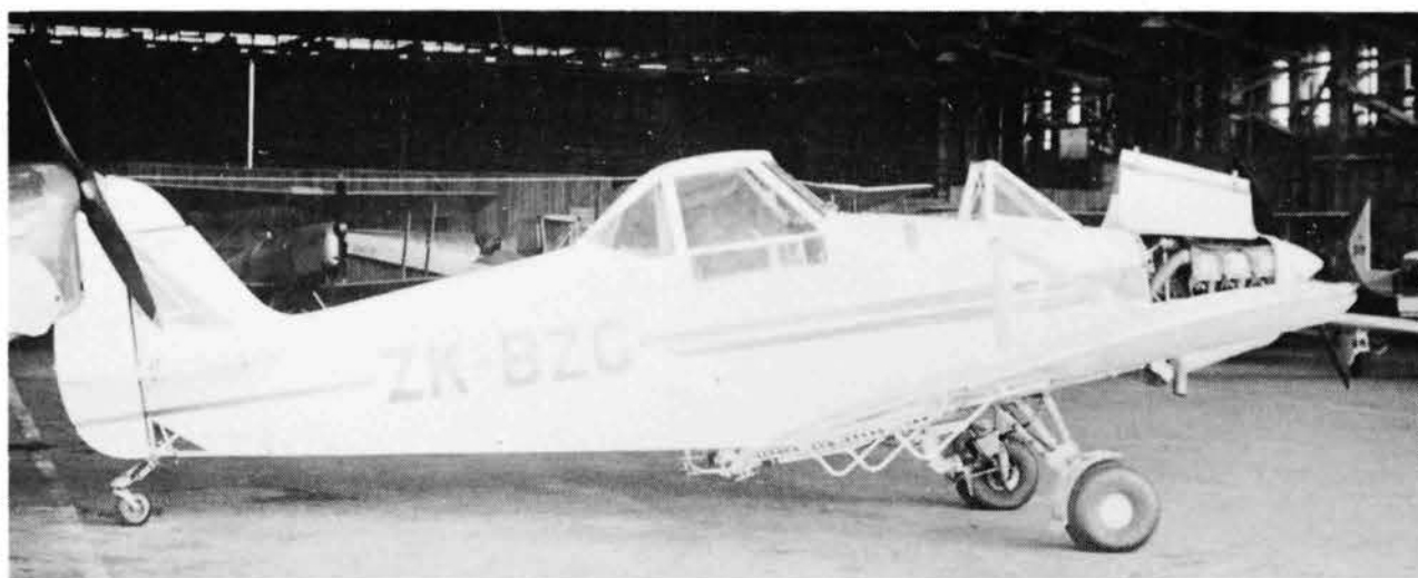
Above: PA-25-235 Pawnee ZK-BZG demonstrates some associated modifications made to the type in New Zealand. To reduce fire risk in accidents, the fuel tanks were moved to the wings and the former tank space together with a small baggage compartment were converted into a passenger "cockpit" for the loader-driver complete with its own angular windscreen. (Wim Zwakhals collection)
