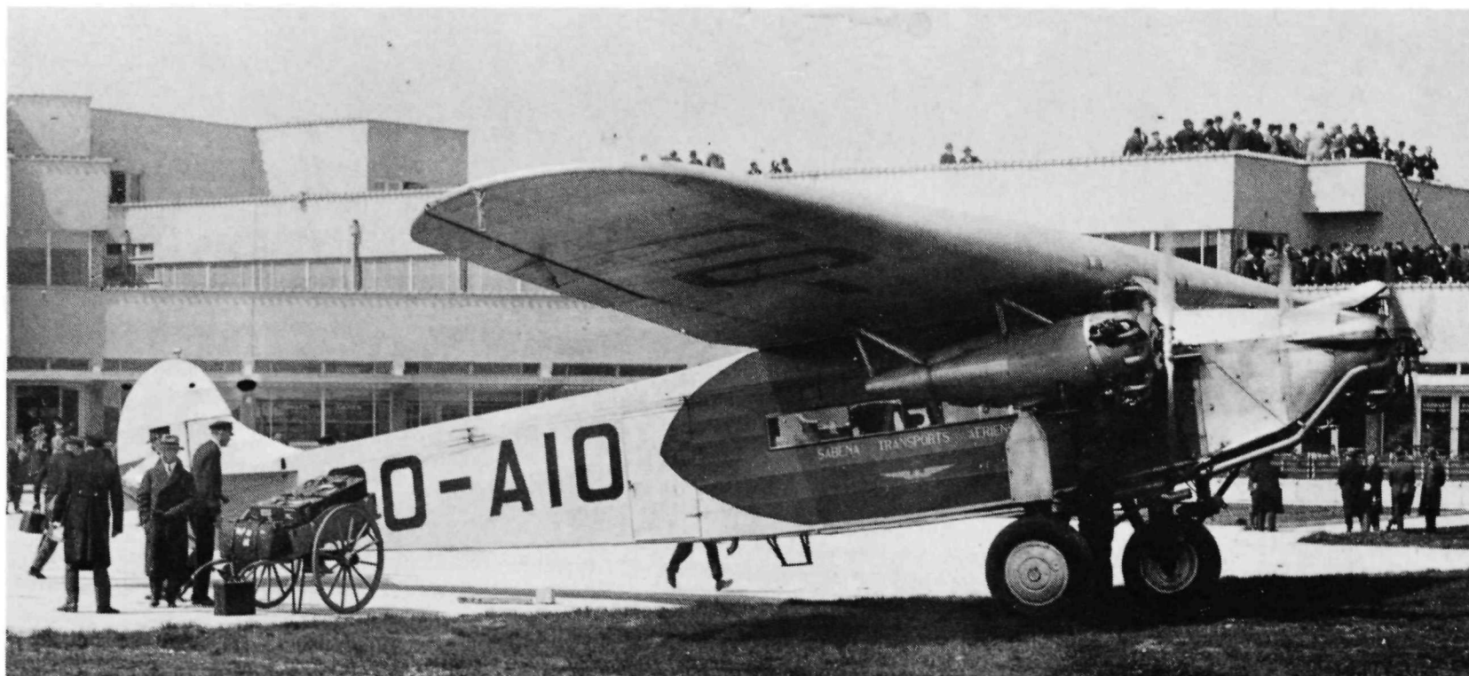
Above: A SABCA-built F.VIIb/3m of SABENA at Antwerp in 1931. OO-AIO shows well the thickness of the cantilever wooden wing, two feet deep at the centre section. Engines of the SABCA-built aircraft were the 230 hp Gnome Rhône-built Bristol 5-cylinder Titans. (via Jack Meaden)
