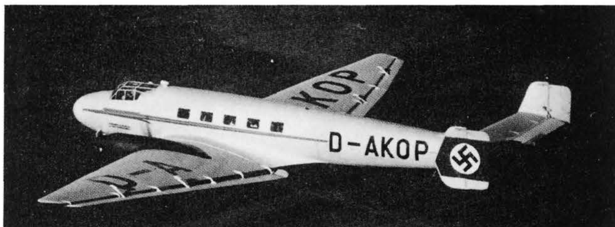
Above: Winner of the Oasis Circuit was D-AKOP, a Junkers Ju 86B-0 with two 600 hp Junkers Jumo 205C diesel engines. The name "Kismet" appeared on the nose and its Competition No.3 was on a white square just behind the registration on the fuselage. (via Jack Meaden)
