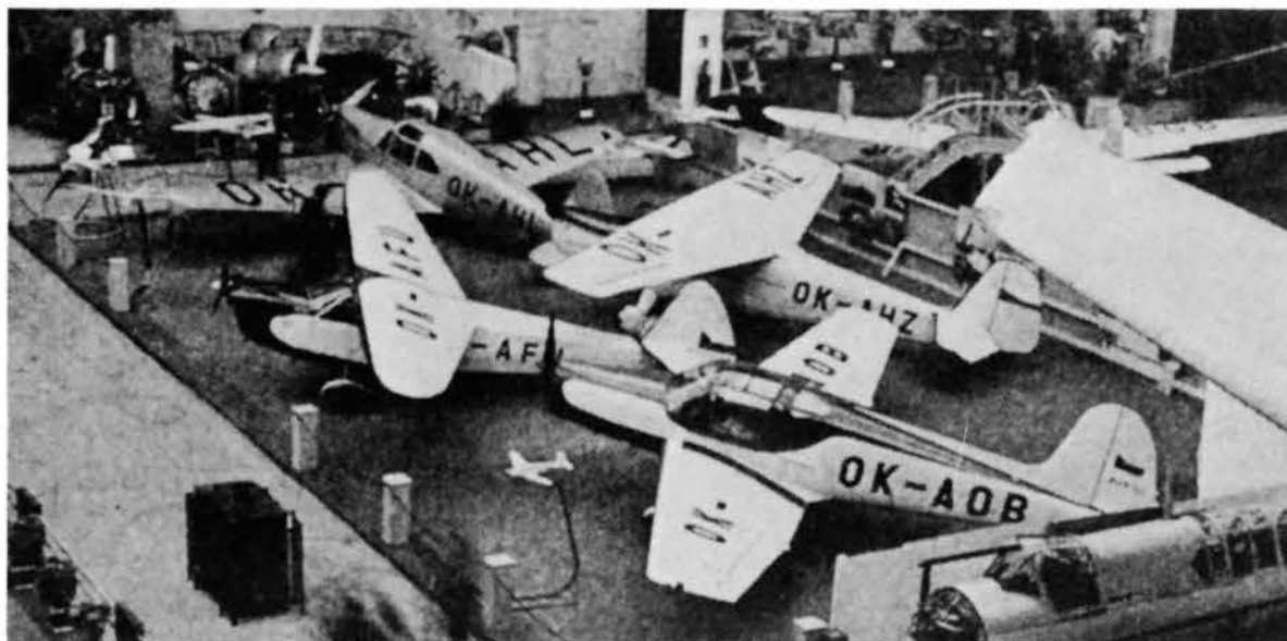
Left: The Czech exhibits are shown in this view with the Zlin 122 OK-AOB and Praga E117 OK-AFU in the foreground. OK-AHZ behind right was the Avia Av.236 Bojar, a 2-seat sportplane of mixed construction with a 4-cyl inverted in-line Walter Mikron III engine giving 65 hp at 2600 rpm. Cruising speed was 99 mph. Behind on the left is OK-AHL, a Mraz Sokol M1C 2-3 seat tourer of wooden construction with retractable undercarriage and 105 hp Walter 4 III Minor. The Sokol was designed clandestinely during the war and flew in 1945. (both Aeroplane via JM) Below: The prototype Zlin 122 OK-AOB was a wood and fabric 3-seat tourer with a Zlin Toma 4-cyl inverted in-line engine giving 94 hp at 2350 rpm at sea level. A clean looking aeroplane with a quoted 119 mph cruise, but it did not enter production.
