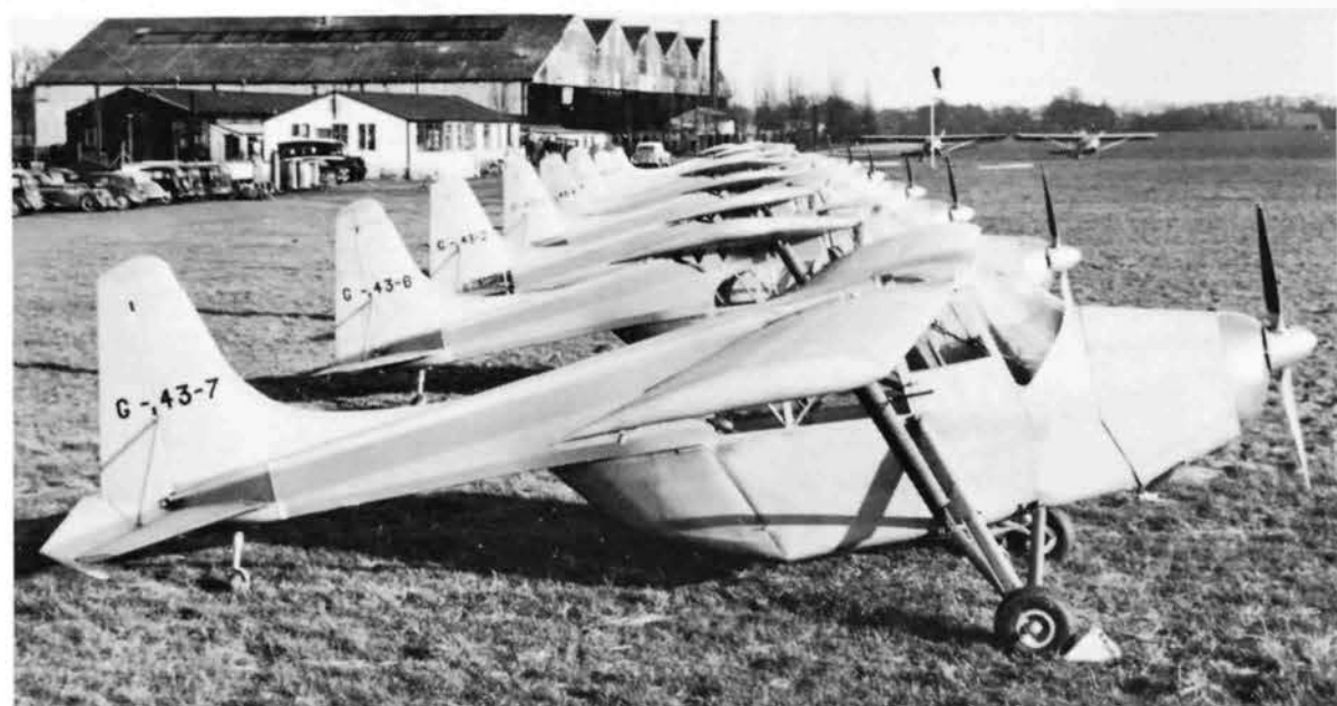
Above: G-APBR c/n 28, ex G-43-7, while still with Edgar Percival Aircraft awaiting sale, is fitted out with spray bars under the wings and a fan-driven pump under the nose. This allowed a 90-foot wide swath to be sprayed from a 170 gallon hopper in the fuselage. (Aeroplane via Jack Meaden)
