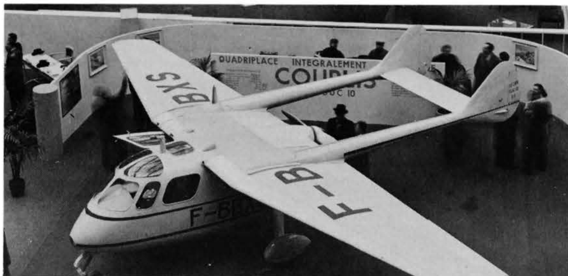
Left: The SUC 10 Courlis in the foreground was a 4-seat all-metal twin boom pusher with a fixed spatted tricycle undercarriage with steerable nosewheel. F-BBXS displayed was the third prototype and the Courlis was already in production with F-BFEQ becoming the 140th production aircraft in due course (although many are thought to have been uncompleted due to problems with the powerplant). The engine was the 200 hp 8-cyl inverted vee in-line Mathis G8R, this giving it an economical cruise of 143 mph, an initial climb of 492 ft/min and a range of 620 miles with a full load of 4 persons. (Aeroplane via Jack Meaden)
