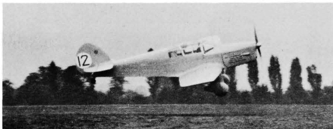
Left: Two views of G-AFAU c/n K.69 which illustrate the two types of windscreen found on the Vega Gull. The upper photograph shows G-AFAU taking off as No.12 during the 1937 King's Cup with the flat-paned sharply tapered windscreen of the Vega Gull Series I.
