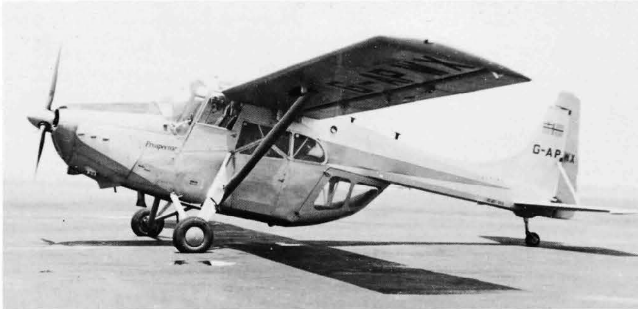
Left: G-APWX c/n 41 was the first LAC Prospector with the 295 hp Lycoming GO-480-G1A6 engine and 3-blade Hartzell c/s propeller. The large rear door windows were fitted for use in locust control in Africa. (John Wegg colln.) Centre upper: G-APWZ c/n 42 wearing Crop Culture (Sudan) Ltd titles 21.9.60 at Lympne. (Jack Meaden) Centre lower: Prospector 2 G-ARDG c/n 47 with 410 hp Cheetah X radial gets airborne at Farnborough in 1960. Bottom: While the Cheetah improved performance it destroyed the important forward view for spraying. (both Aeroplane via Jack Meaden)
