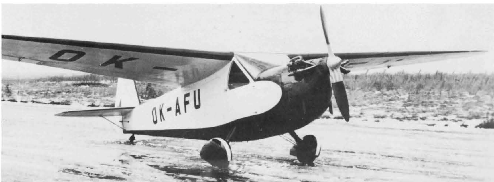
Above: The second prototype Praga E117 OK-AFU which was displayed (top) with a 79 hp 4-cyl horizontally opposed Praga D engine. The E117 was a postwar development of the E114 which was built in the UK pre-war as the Hillson Praga by F. Hills & Sons. The E117 structure was updated, the wooden fuselage replaced with fabric-covered welded steel tube, the cantilever wooden wing lost its straight centre-section in favour of straight taper, and flaps were added. Cockpit doors replaced the open up and fold down hinged entry and the cabin was more spacious. (Jack Meaden) Left: A model was displayed of the Czech Avia 38A, a light alloy stressed-skin twin-boom 5-seat cabin monoplane with two 160 hp Walter Minor 6-III engines geared to drive contra-rotating pusher propellers. It was said to have had a retractable tricycle undercarriage, but nothing more was heard of it. (via Jack Meaden)
